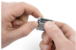
Open the Gelbox at the side latches.
